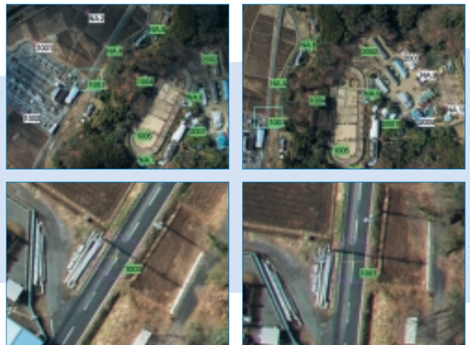
Determining and measuring common points for bundle adjustment
